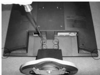
1. After placing monitor on the cushioned table, remove 6 screws on the left and right of the bottom.
